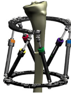
Figure 7a Proximal 2/3 Ring with 180° Rotary Offset combined with Custom Strut Mount on the Distal Ring to maximize the window over a wound
