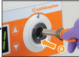
Insert pump cartridge into console
