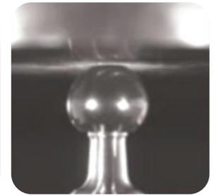
Top-load comparison of monolithic alumina ceramic (top) and OXINIUM femoral head (bottom).<sup>28</sup>
