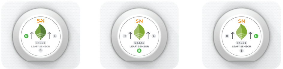
Figure 10: LEAF Patient Sensor LED scrolling pattern
