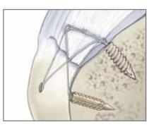
STEP 6: Establish and maintain axial alignment of the suture anchor to the prepared insertion site, and place the tip of the anchor into the prepared hole. Using a mallet tap the FOOTPRINT Ultra PK suture anchor inserter handle until the laser mark is flush with the cortical bone.
