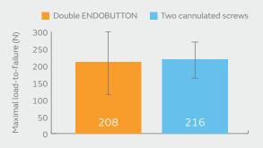
Figure 1. Average maximal load to failure (± standard deviation)
