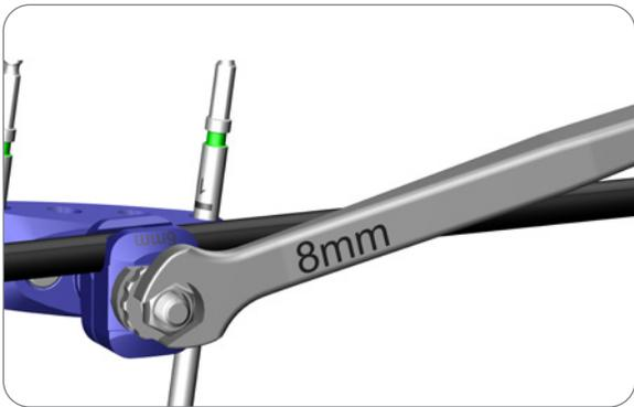
Check the frame to ensure that all tightening points on the clamps are locked.
