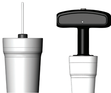
Correct drill or punch hole depth
