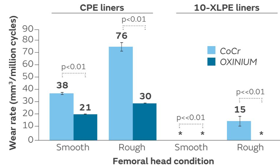
Figure. Wear rate of CPE and 10-XLPE liners against CoCr and OXINIUM femoral heads under smooth and roughened conditions
