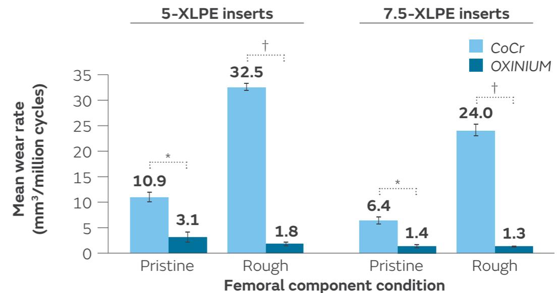
Figure. Wear rate of 5-XLPE and 7.5-XLPE tibial inserts against OXINIUM and CoCr femoral components
