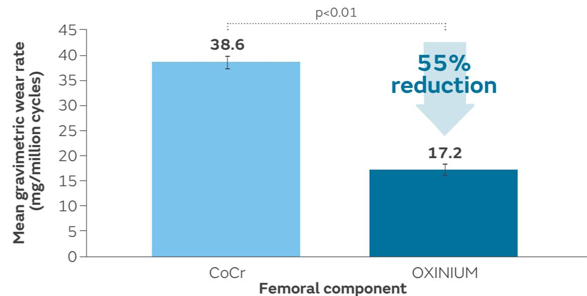
Figure. Mean gravimetric CPE wear rate with CoCr and OXINIUM femoral components
