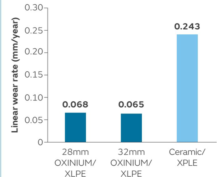
Figure 2. Linear wear rate of OXINIUM and ceramic femoral heads articulated against XLPE liners
