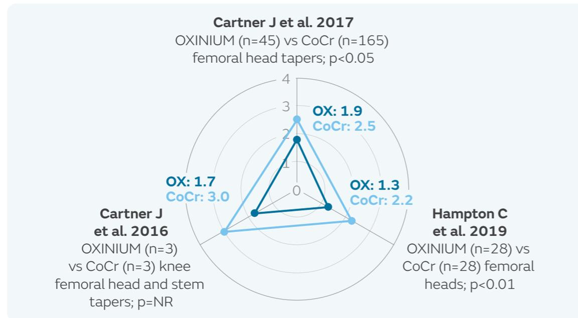
Figure 1. Mean Goldberg corrosion scores for retrieved OXINIUM and CoCr components across three studies
