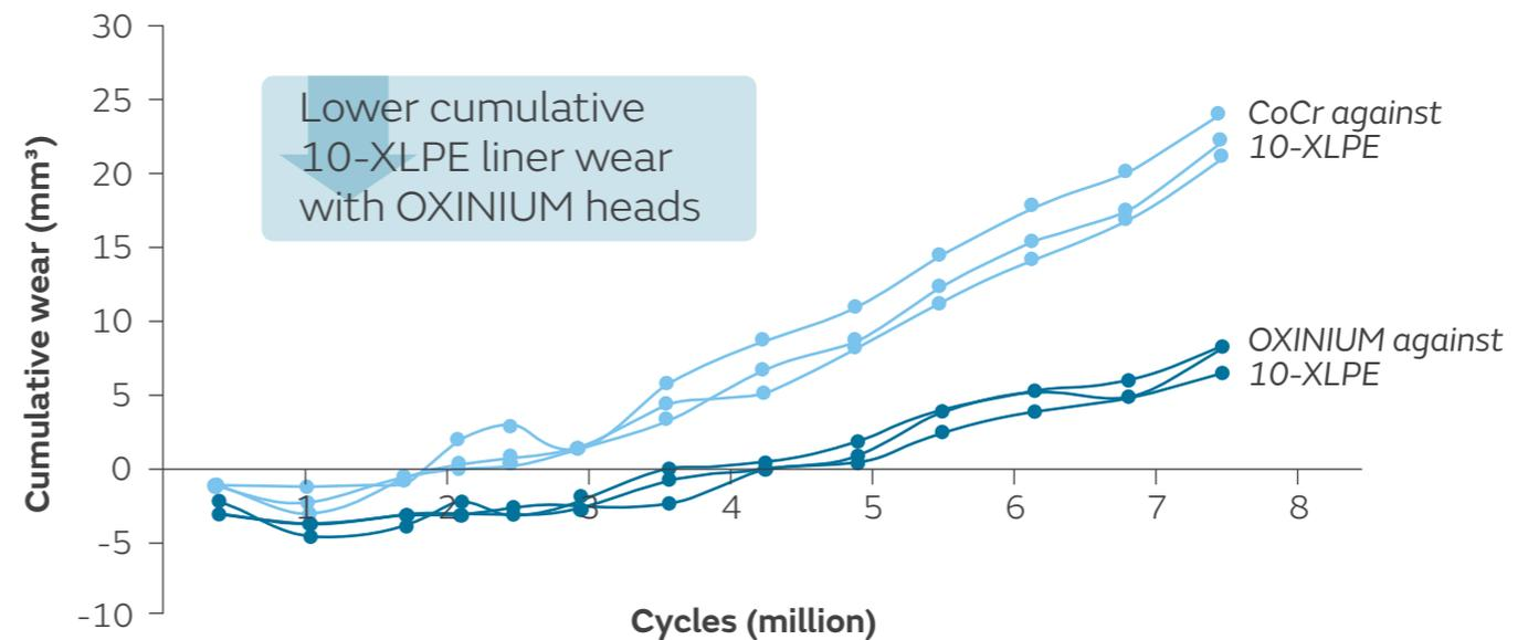
Figure. Cumulative wear of 10-XLPE liners articulated against 36mm OXINIUM and CoCr heads
