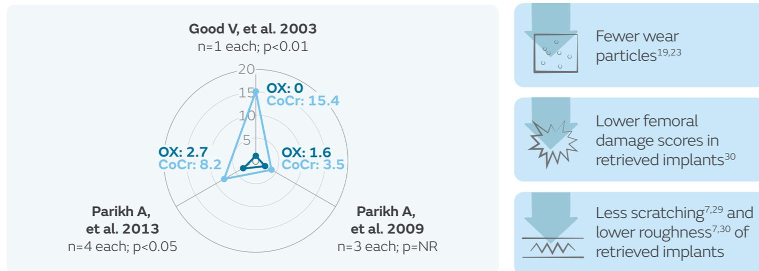
Figure 1. Wear rate (mm<sup>3</sup>/million cycles) of OXINIUM and CoCr femoral heads articulated against highly cross-linked polyethylene (XLPE) liners
