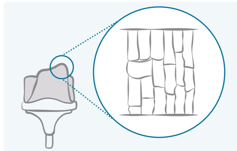
Figure. Columnar arrangement of OXINIUM oxide layer and features that may confer its surface durability
