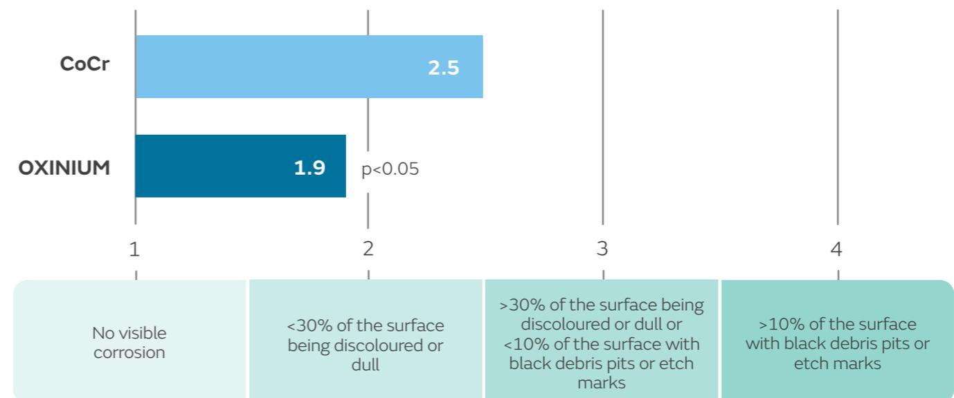
Figure. Mean corrosion score of retrieved CoCr and OXINIUM femoral heads
