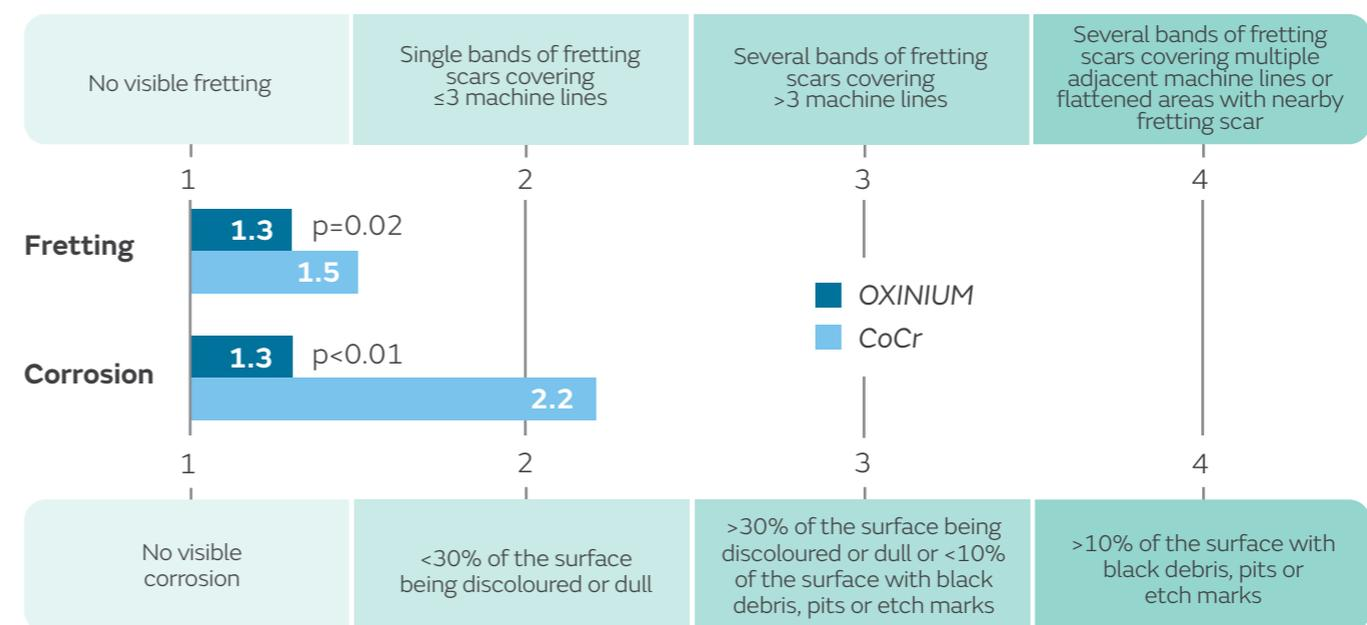
Figure. Mean fretting and corrosion scores of retrieved CoCr and OXINIUM femoral heads
