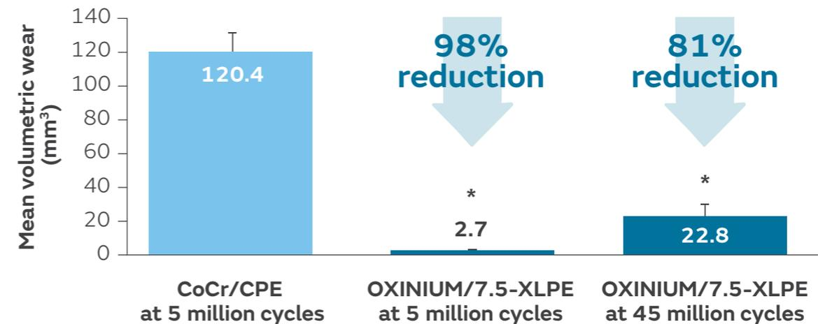
Figure. Mean volumetric wear of CoCr/CPE and OXINIUM/7.5-XLPE couples
