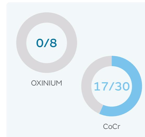
Figure 2. Proportion of retrieved OXINIUM and CoCr femoral heads with Goldberg corrosion scores >3 that exhibited material loss due to MACC
