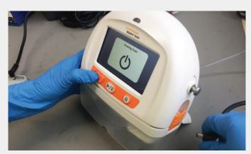
1. Turn off the device and disconnect from mains power before cleaning and disinfecting to prevent electric shock.
