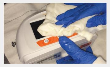
Wipe down the surface of the device with a soft cloth dampened with cleaning agent or an impregnated disposable wipe. Use a neutral pH7 detergent/disinfectant or antimicrobial agent that is safe to use with plastics.
