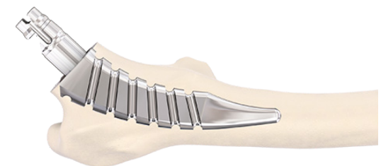
Figure 17: Compactor in situ
