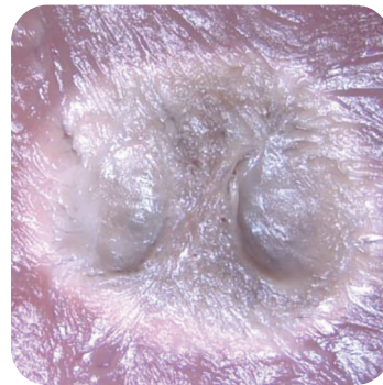
Figure: Typical appearance of FASTSEAL 6.0 (left) and monopolar electrocautery device coagulation treatments in bovine myocardium (beef heart) soft tissue model. 8 (right)
